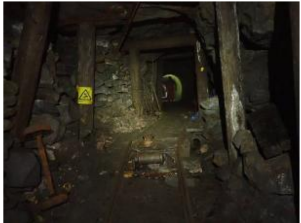
Top of the final incline. Note reused electricity pole
